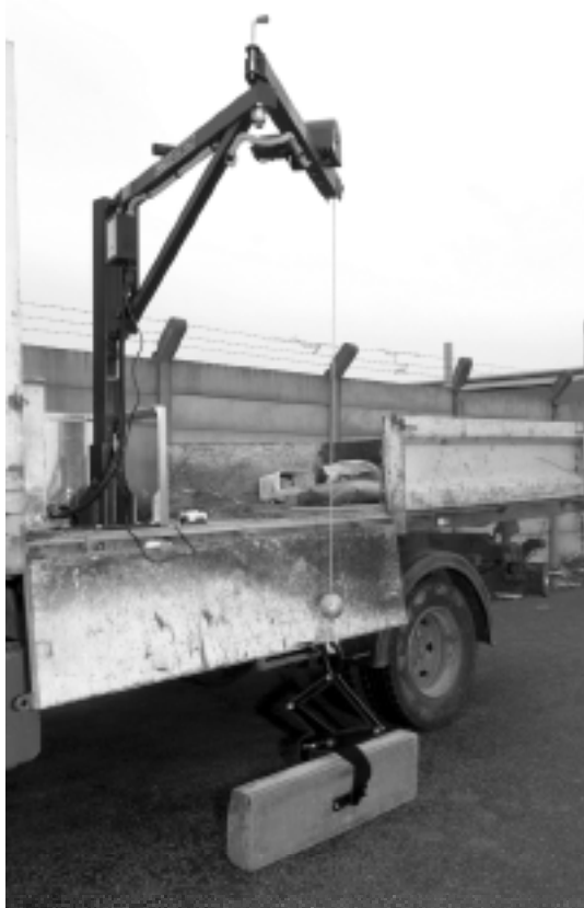
Figure 2 Vehicle-mounted crane and mechanical grab
